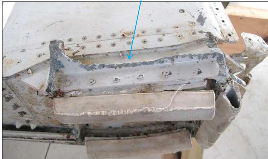
Lower surface side hinge fitting fracture
