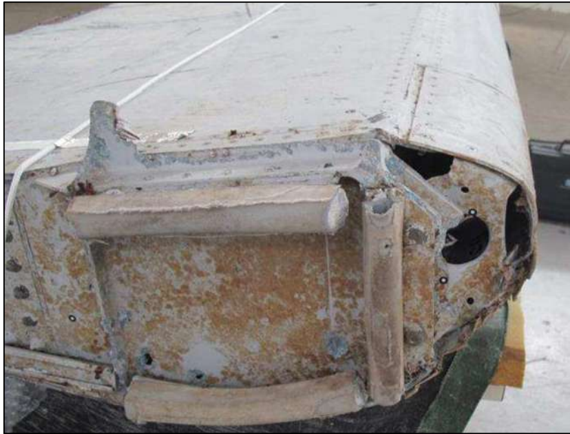
Disassembly of leading edge panel
