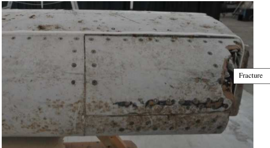
Fracture of the access door on the inboard side
