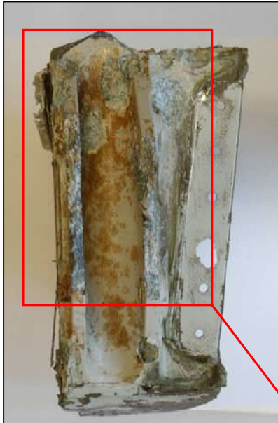
Planche 39 : Leading edge side inboard hinge fitting fracture
