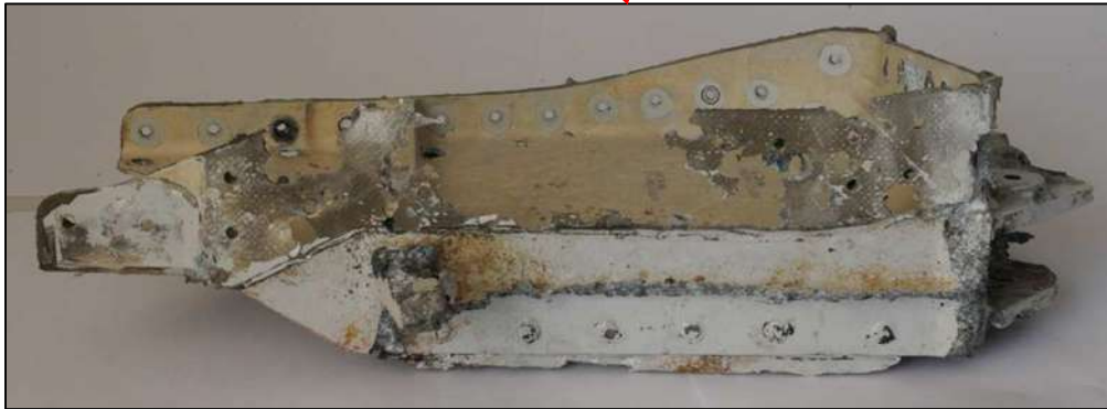
Lower surface fracture
