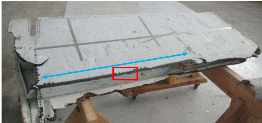
Planche 52 : Lower surface: straight fracture on trailing edge
