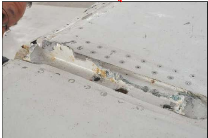
Lower surface fracture
