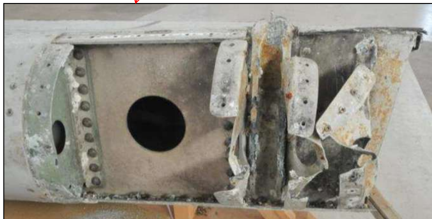
Leading edge fracture
