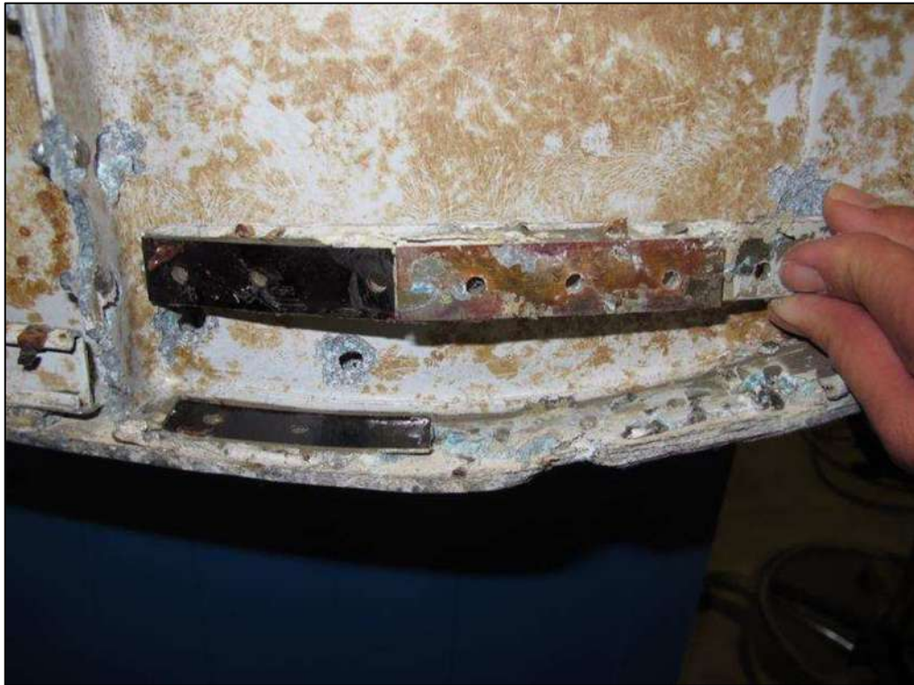
Repair: disassembly of seal retainer
