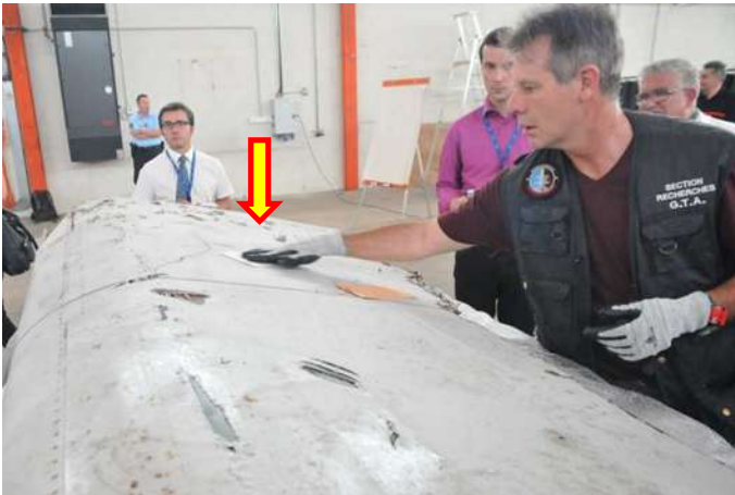
Sampling to search for explosive residues
