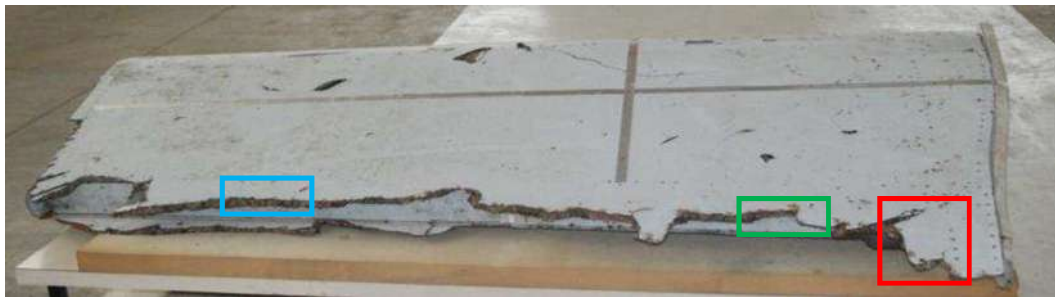
Regular fracture, without protruding fibres
