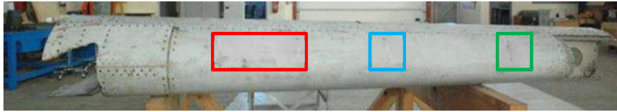
Planche 47 : Impacts on the leading edge
