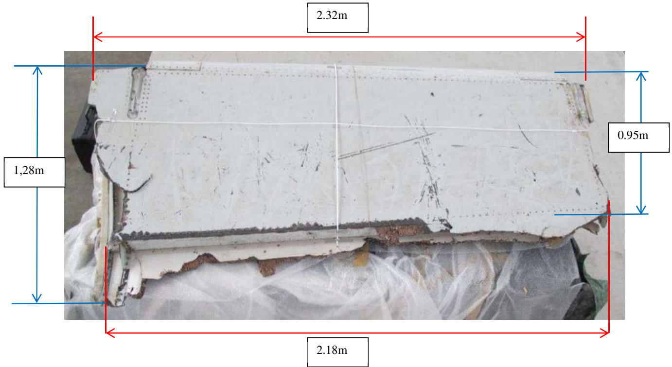
Planche 18 : Dimensions and position of the centre of gravity lower surface side
