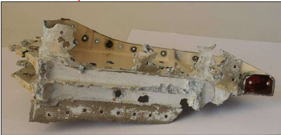
Lower surface fracture
