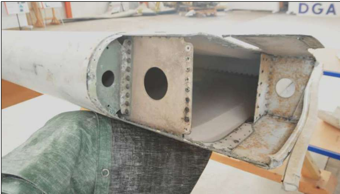
Planche 26 : View of the flaperon after disassembly of the outboard hinge fitting
