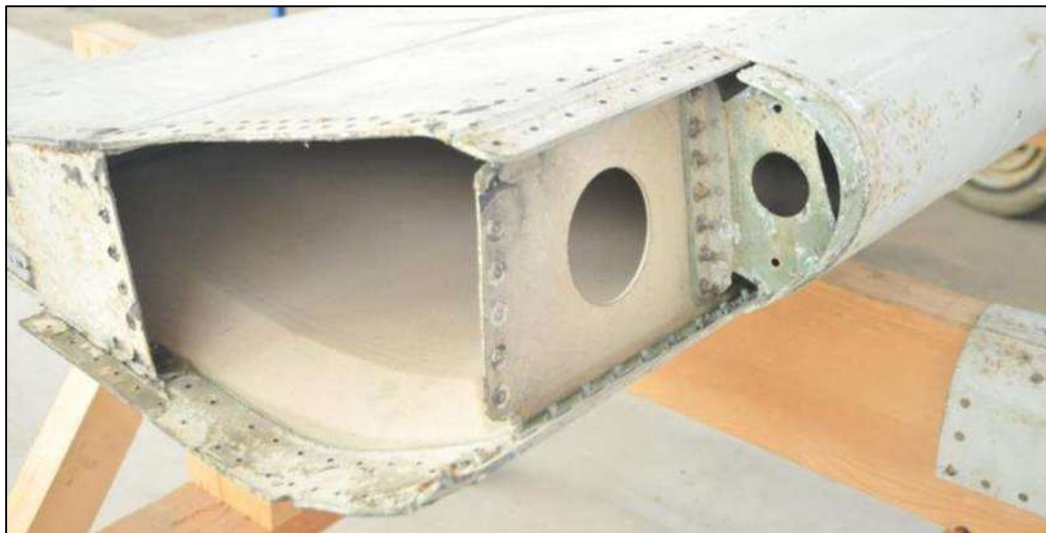
Lower surface side hinge fitting fracture
