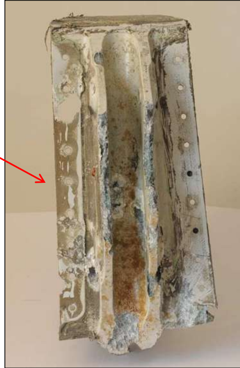
Leading edge fracture
